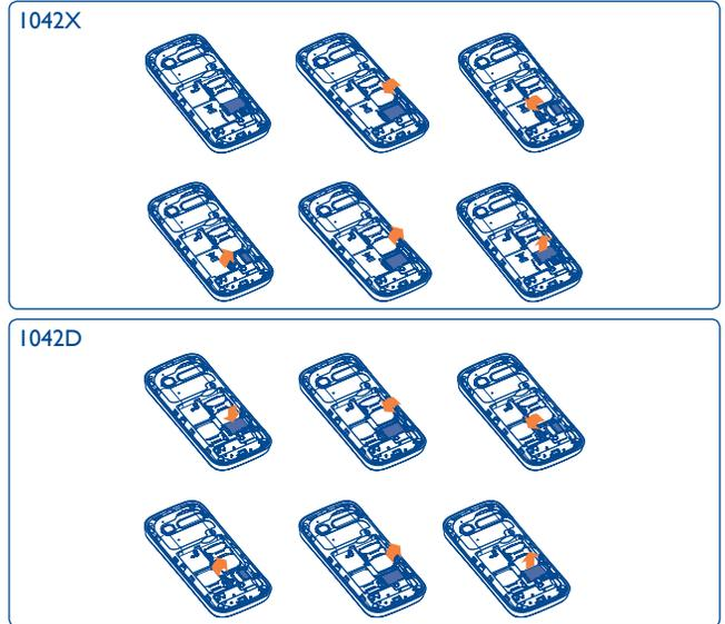
To release the microSD card holder, slide it in the direction of the arrow and lift it. Then insert the microSD card with the golden contact downward. Finally, turn down the microSD holder and slide it in the opposite direction to lock it.
