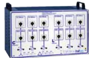
MOD4020-LC110T Charge for triphase alternator • Inductive & capacitive load variable with 3x 1%÷110%; • 3Ph: variable with 110 steps from 1% to 110% • Power: 10÷1000VA; Triphase / monophase; (monophasé with 330 steps);
