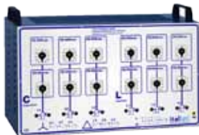
MOD4020-LC20T Load for 3-phase alternator Load inductives & capacitives; Variable with 20 steps : 5% ÷100%; Power: 50VA÷1000VA Triphase / monophase; (monophasé with 60 steps);
