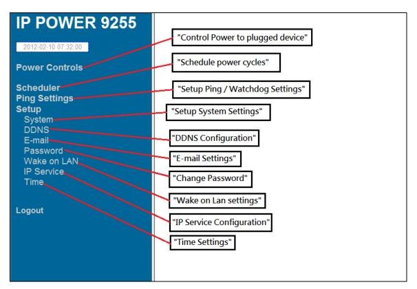
**Power Controls:** Turn off, Turn on, the socket to provide power to the device. **Scheduler:** Schedule specific dates or time to call an action to the IP Power 9255.
