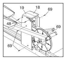
removed from; the Screws will later need to be reattached in the same holes. Carefully separate and remove the Flywheel Covers.
