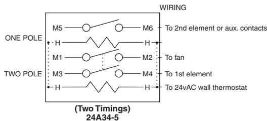
..... DOTTED LINE BETWEEN "H" TERMINAL IS A FACTORY-INSTALLED JUMPER
