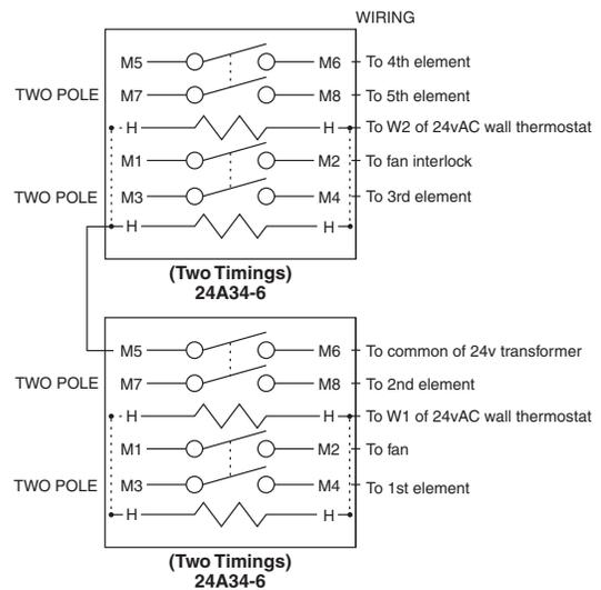
..... DOTTED LINE BETWEEN "H" TERMINAL IS A FACTORY-INSTALLED JUMPER
