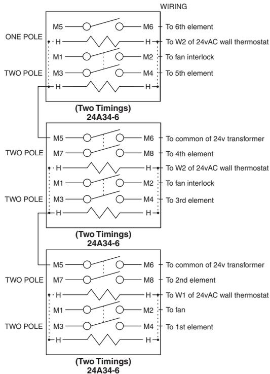
..... DOTTED LINE BETWEEN "H" TERMINAL IS A FACTORY-INSTALLED JUMPER
