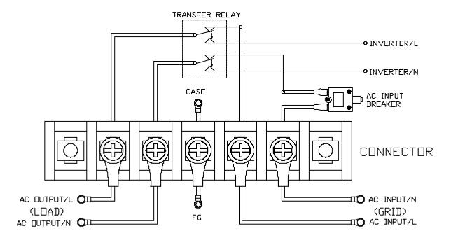
■ Connect AC output and AC input wiring to the Inverter terminals.
