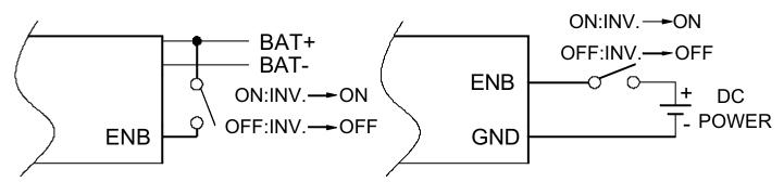
NOTE: At one time, only one remote function should used to control the inverter. The maximum voltage value is the same as input DC voltage.
