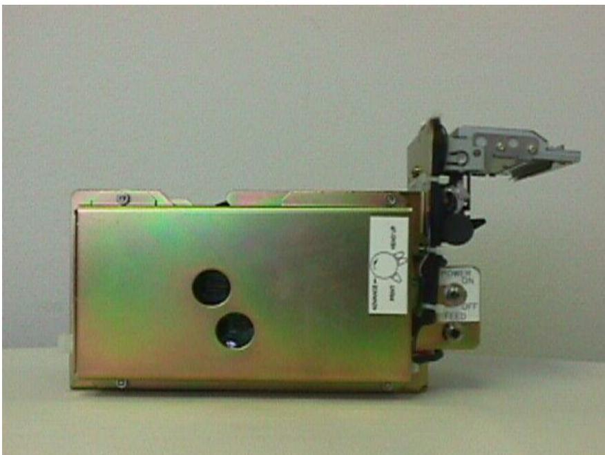
*Figure 6 - MTP-640 with Cutter Mechanism open*
