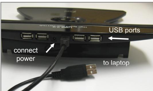
After the connections in step 1 are completed (be sure to follow correct order) you can begin connecting your USB devices to the Station's integrated USB ports.
