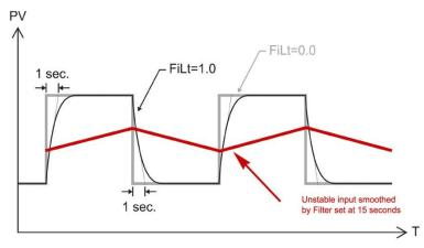
uncontrollable. Set the time constant for the digital filter (the first order filter) depending on how unstable the input is. The example below shows the result when no filter is used, when a 1 second and finally 15 second filter is used.
