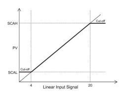
The Cut-off function is used to limit the input signal display (PV) within the limits defined by the user whenever the input signal is out of the scale defined by  $\frac{SERL}{L}$  and  $\frac{SERH}{L}$ . The cut-off function can be set to "Low", "High" or "High/Low" or set to "None" to disable it. The cut-off function has no effect for input signals other than linear types and is only showed when the input signal type is set to linear.
