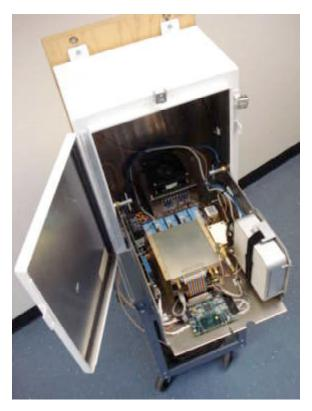
The transceiver generates and transmits the RiverSonde signal. It also receives and conditions the reflected signal. It communicates with the processor, receiving commands and forwarding received signal data. It sends measurement signals to and receives reflected signals from the antenna. The transceiver is housed in the enclosure. The photo above shows the transceiver electronics mounted in the enclosure. A schematic diagram of the transceiver is shown below.
