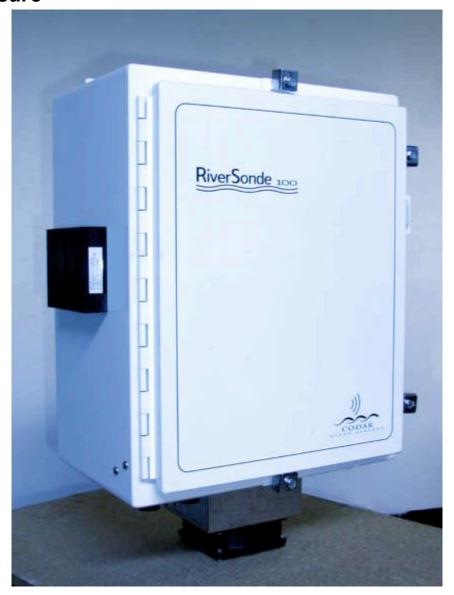
The enclosure provides weather-resistant protection for the transceiver and the processor. In addition, the enclosure is outfitted with a self-contained air conditioner that cools the enclosed electronics. A door with a weather-resistant seal allows access to the enclosed transceiver and processor. It has external connectors for power, communication and antenna signals. The enclosure is mounted to the antenna mast.
