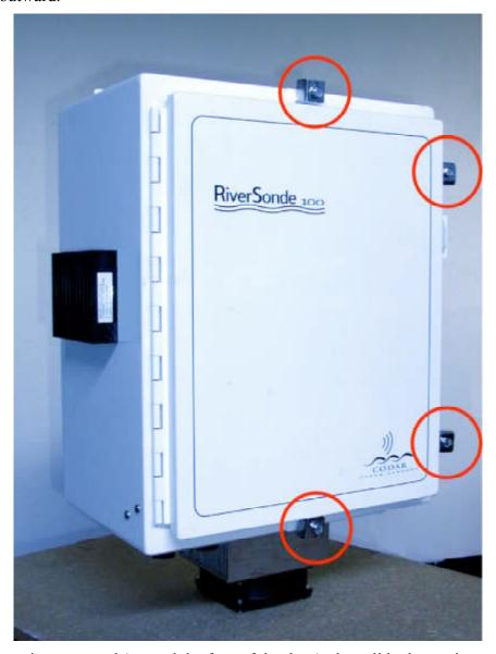
Pull each retainer outward (toward the face of the door), then slide the retainer away from the lip on the door's edge.
