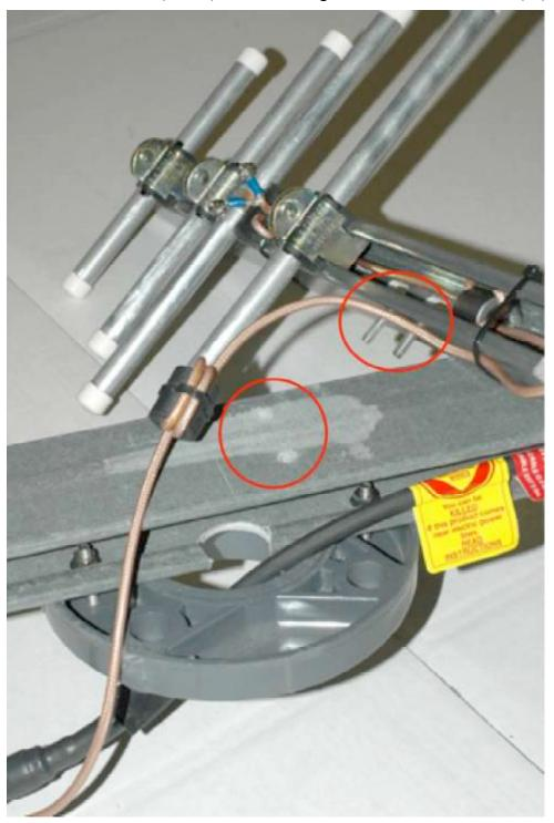
Attach center antenna to cross member, tighten nuts.
