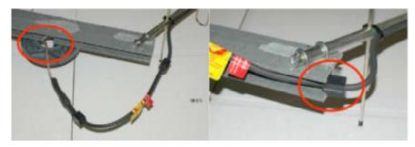
Feed the remaining cable from the #3 antenna under the center antenna rail and into the center hole of the flange.
