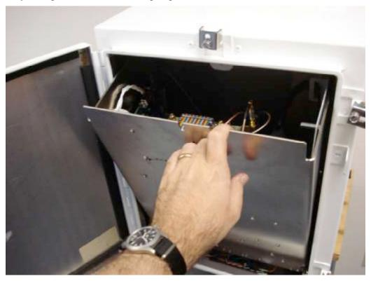
There are two spring plungers at the rear of the bracket (as you face the door). Rotate each spring plunger handle 90 degrees to extract the plunger.
