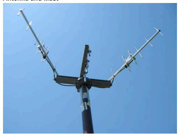
The antenna transmits signals from the transceiver to the river. It also receives reflected signals from the river. Each of the three antenna elements is connected to the transceiver by a cable. The antenna is mounted on top of a hollow fiberglass mast. The mast is secured on the ground with a user-provided post.
