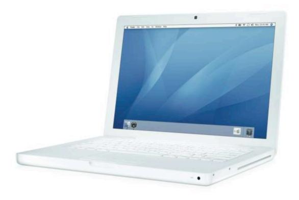
The interface computer is a portable computer, outside the enclosure, used to set up, configure and control the RiverSonde. It is also the user interface to the RiverSonde, communicating with the processor via the *RSCommander* program. Use the interface computer to view and download data summaries, request plots and configure the RiverSonde. The interface computer communicates with the processor via a local wired Ethernet connection, an optional wireless connection, or an Internet connection.
