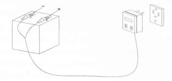
When the green LED light is on, disconnect the charger from the battery terminal and the wall outlet. If the green LED light does not come on after 10 to 12 hours of charging time or the green LED light comes on relatively soon after the charger is plugged in, this may indicate that the battery will not accept a full charge. If this occurs and also your camera run time is greatly diminished, you may need to replace with a new battery of equal specification.
