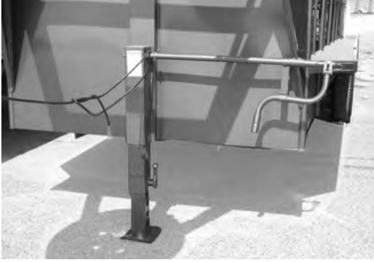
Drop Leg Mechanism
