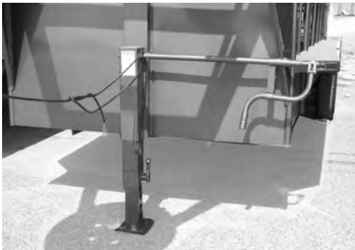
Drop Leg Mechanism
