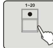
9. Press the number button **1-20** to select the Override number you chose in step 2, all LEDs blink for 3 times to indicate that you have successfully edited an Override effect.
