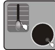
3. Move **FADERS1-24** to vary the channel outputs or use Jog wheel **#1**、**#2** to adjust PAN and PAN FINE or use Jog wheel **#3**、**#4** to adjust TILT、TILT FINE.
