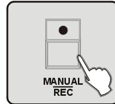
4. Once the effect is adjusted, press **MANUAL/REC** button to store, at this moment, all LEDs on **CUE**、**OVERRIDE**、**CENTER**、**FIXTURE GROUP**、**PRESET**、**CHASE**、**BANK**、**BLACKOUT** blink at the same time.
