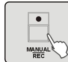
5. Press **MANUAL/REC** Button, at this moment, all LEDs on **CUE**, **OVERRIDE**, **CENTER**, **FIXTURE GROUP**, **PRESET**, **CHASE**, **BANK**, **BLACKOUT** blink at the same time.
