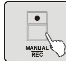
6. Press **MANUAL/REC** button, at this moment, all LEDs on **CUE**, **OVERRIDE**, **CENTER**, **FIXTURE GROUP**, **PRESET**, **CHASE**, **BANK**, **BLACKOUT** blink at the same time.
