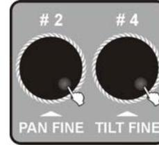
3. Use Jog wheel **#2** and **#4** to change the name of the FIXTURE. Turn Jog wheel **#2** to change the position of the cursor, and Jog wheel **#4** should be used to change the trait of the channel or character. The amount of the letters must be below 26, it can be include ten numbers, one “—”, the length of the Fixture name should be below 16, and it must be begin with letter.
