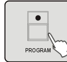
10. Press **PROGRAM** button for 3 seconds to exit Program mode, the LED goes out indicating this operation.
