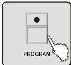
9. Press **PROGRAM** button for 3 seconds to exit Program mode, the LED goes out indicating this operation.
