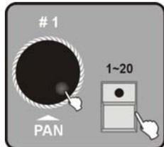
3. Press the number button **1-20** to select the to be stored CUE number, at this moment, all LEDs on CHASE are lit and all LEDs on the number button which have saved CHASE will blink. Turn jog wheel **#1** should change the page number.
