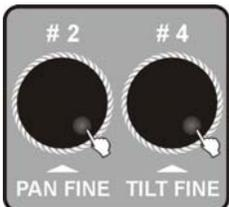
5. Use Jog wheel **#2** and **#4** to change the name of the FIXTURE. Turn Jog wheel **#2** to change the position of the cursor, and Jog wheel **#4** should change the trait of the channel. The amount of the letters must be below 26, it can be include ten numbers, one "—", the length of the Fixture name should be below 16, and it must be begin with letters.
