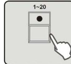
7. Press the number button **1-20** to select the location to store the Center all LEDs blink for 3 times to indicate that you have successfully stored a Center position.
