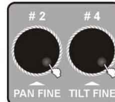
7. Use Jog wheel **#2** and **#4** to change the name of the FIXTURE. Turn Jog wheel **#2** to change the position of the cursor, and Jog wheel **#4** should change the trait of the channel
