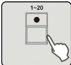
9. Press the number button **1-20** to select the location to store the Center, all LEDs blink for 3 times to indicate that you have successfully edited a Center position.
