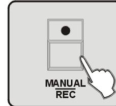
7. Press **MANUAL/REC** button, at this moment, all LEDs on **CUE**, **OVERRIDE**, **CENTER**, **FIXTURE GROUP**, **PRESET**, **CHASE**, **BANK**, **BLACKOUT** blink at the same time.
