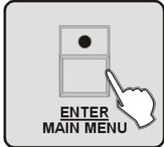
6. Press **ENTER/MAIN MENU** Button, all LEDs shaking for 3 times means success.
