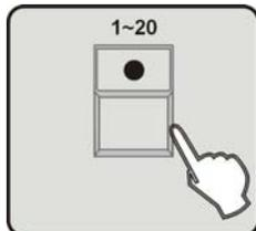
4. Press the number button **1-20** to select the Chase number which is to be stored to CUE, the LEDs on the chosen number buttons will be lit.
