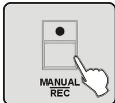
5. Press **MANUAL/REC** button, all LEDs blink for 3 times to indicate that you have successfully stored a CUE.
