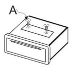
Note: Remove the protection screws (A) before installing and operation the unit.
