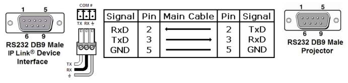
Note: Captive screw connector may also be used as a serial connection.
