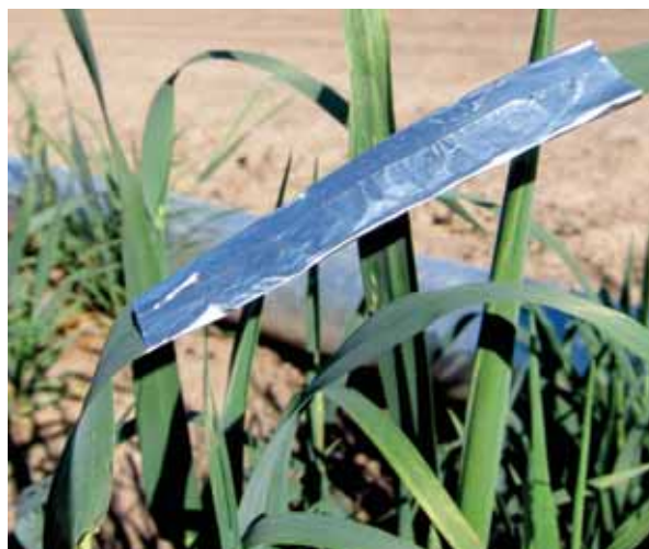
Figure 13.3. A self-made dark adaptation leaf clip using aluminum foil.
