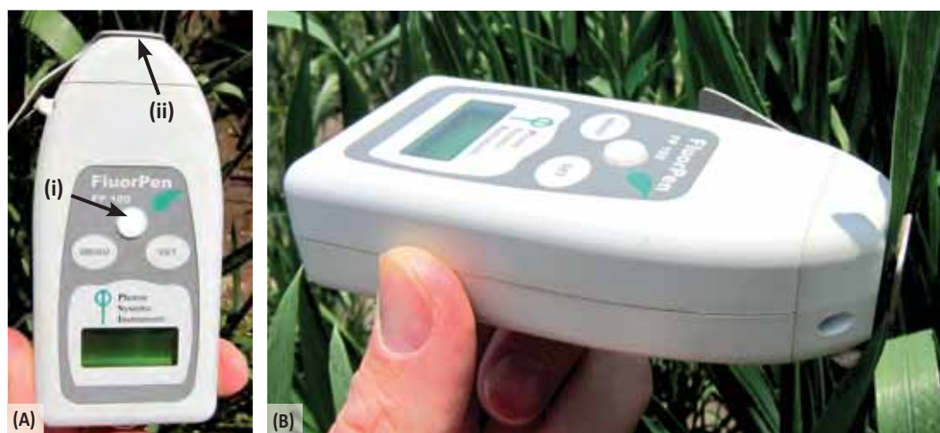
Figure 13.2. Hand held chlorophyll fluorometer Fluorpen FP-100: (A) showing (i) PAR sensor, and (ii) sample leaf in sensor chamber; (B) field measurements in daylight conditions.
