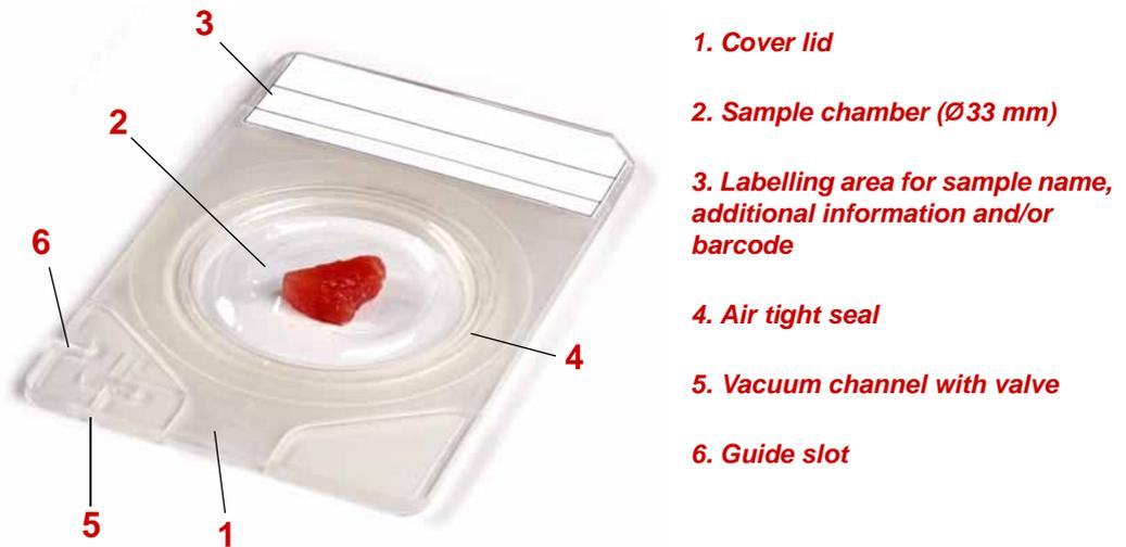
Figure 9. Main parts of Maintainor card.
