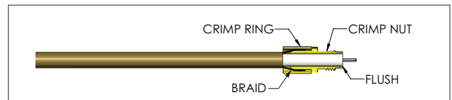
Figure C. Apply threaded crimp nut; ensure the end of the dielectric is flush with the end of the threaded crimp nut.
