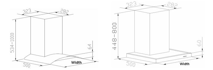
BR603CPX, BR603CPX-F, Width=600; BR903CPX, BR903CPX-F, CRHC9S01-1, CRHC9S01-F, Width=900
