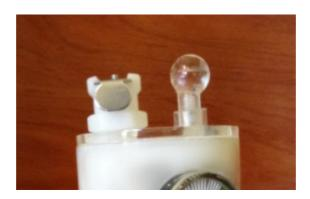
To the left of the photo is the white connector which connects to the cylinder, to the right of the **air** release valve. The pump is sold with standard male and female connectors suitable for many types of tubing.
