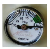
The analog vacuum gauge, measures " $^{\circ}$  Hg (inches of mercury), the green part ie 5 to 10 is a range considered high for static pumping.
