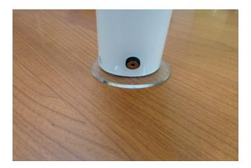
The connector to recharge the internal battery is located behind in the lower part of the device.
