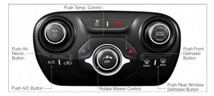
For your convenience the climate controls can be operated by using the soft-keys located on the touch-screen or the climate control knobs below the Uconnect<sup>®</sup> touch-screen.
