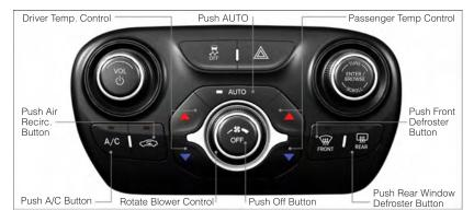
For your convenience the climate controls can be operated by using the soft-keys located on the touch-screen or the climate control knobs below the Uconnect<sup>®</sup> touch-screen.
