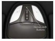
Erase all channels before you begin programming. To erase the channels, place the ignition switch into the ON/RUN position, then press and hold the two outside HomeLink<sup>®</sup> buttons (I and III) for up to 20 seconds or until the red indicator flashes.
