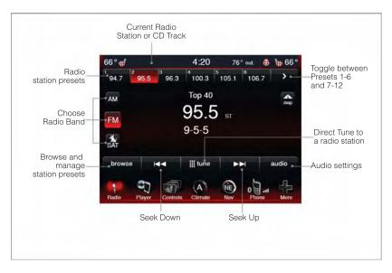
• To access the Radio mode, touch the Radio soft-key at the lower left of the screen.
