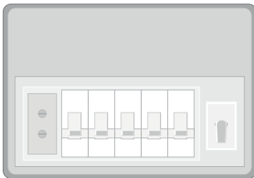
Trip switch: replaces fuses in modern fuse boxes
