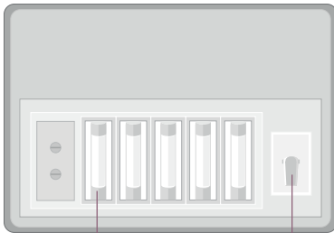
Electricity Consumer Unit (fuse box)
