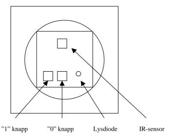
The main components on the PCB are two programming buttons ("1" knapp, "0" knapp), one LED (Lysdiode) and a IR-sensor on the PCB.
