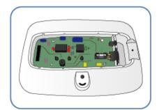
► Open the cover as Fig. then you can see fuse equipped PCB. Remove failure fuse with screwdriver.
