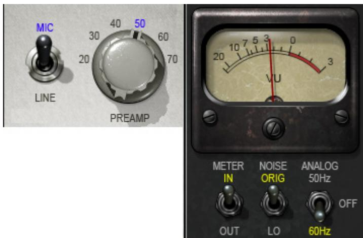
To control analog coloration, use the Source switch to select Mic/Line amplification and the Preamp knob to select the amount of coloration. Higher values introduce more harmonic distortion with increased noise and hum. The overall level will not change significantly, as the HLS recreates the coloration alone, not the amplification itself.
