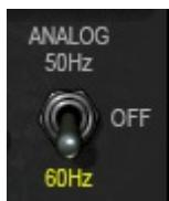
**Analog** controls turns the analog noise and hum modeling on and off, and sets the pitch of the hum to match either European or American currents. To retain only the modeled harmonic distortion, bypass the noise and hum by setting Analog to Off.
