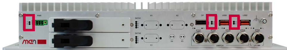
Figure 16. Status and user LEDs on the BL50S's front panel (highlighted in red)
