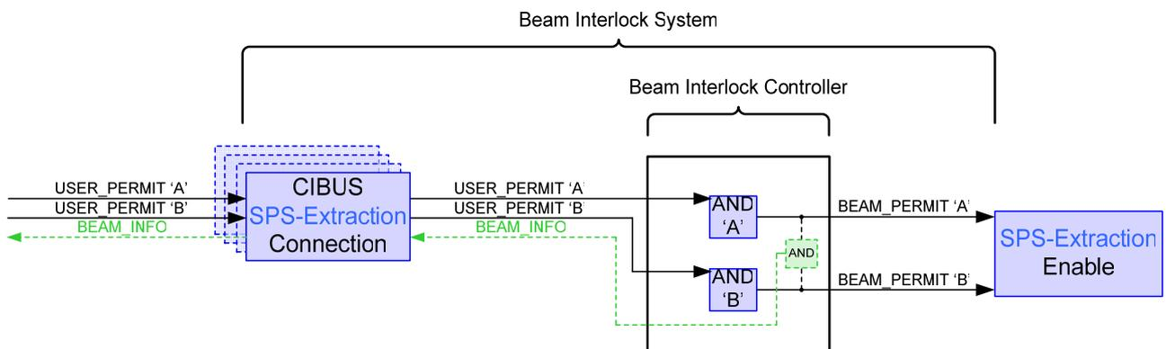
Figure 3: Simplified Architecture of SPS Extraction and Transfer Lines Interlock System
