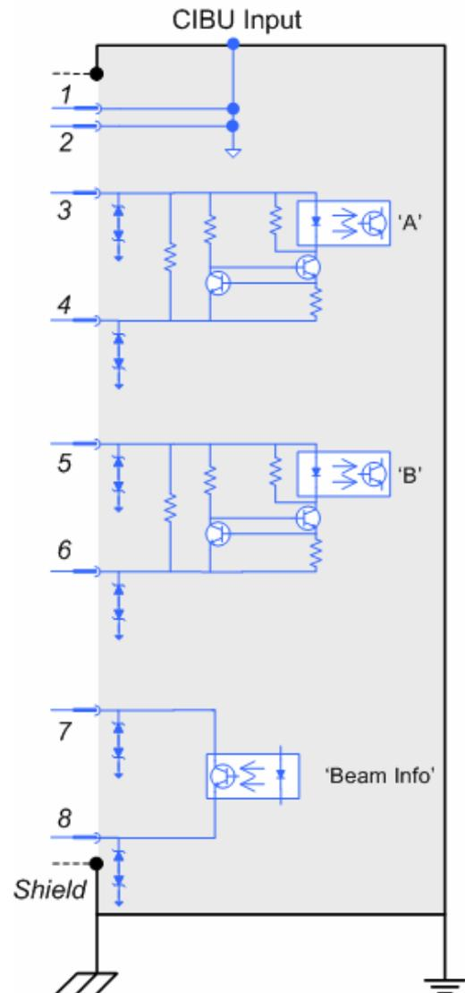
Figure 11: CIBU Input Circuit Schematic
