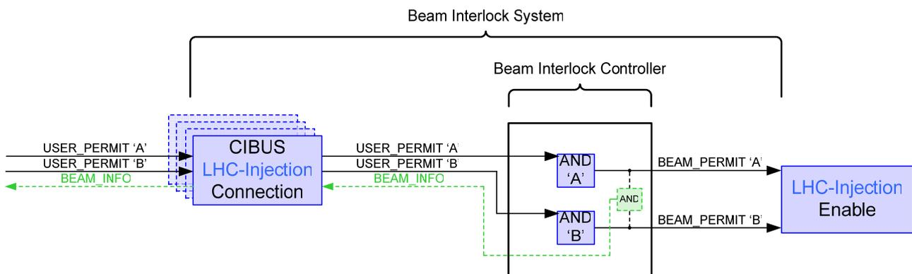
Figure 4 : Simplified Internal Architecture of the LHC Injection Interlock system
