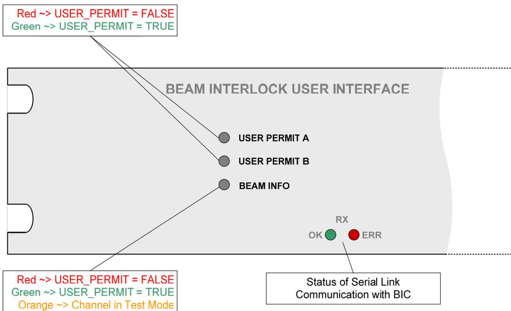
Figure 8: CIBU Tri-Colour Light-Emitting Diode Function
