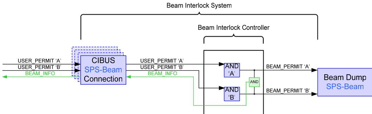
Figure 2: Simplified Internal Architecture of the SPS Beam Interlock System
