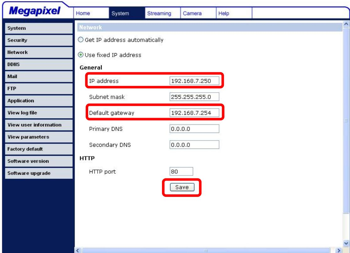
The screenshot shows the Megapixel web interface with the 'System' tab selected. The 'Network' section is active, and the 'Use fixed IP address' option is selected. The 'General' section contains the following fields:
