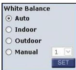
A digital camera needs to find reference color temperature, which is a way of measuring the quality of a light source, for calculating all the other colors. The unit for measuring this ratio is in degree Kelvin (K). Users can select one of the White Balance Control modes according to the operating environment. The following table shows the color temperature of some light sources.
