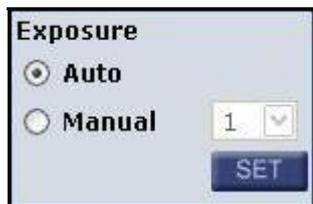
The exposure is the amount of light received by the image sensor and is determined by the width of lens diaphragm opening (iris adjustment), the amount of exposure by the sensor (shutter speed) and other exposure parameters. With this item, users can define how the Auto Exposure function works.
