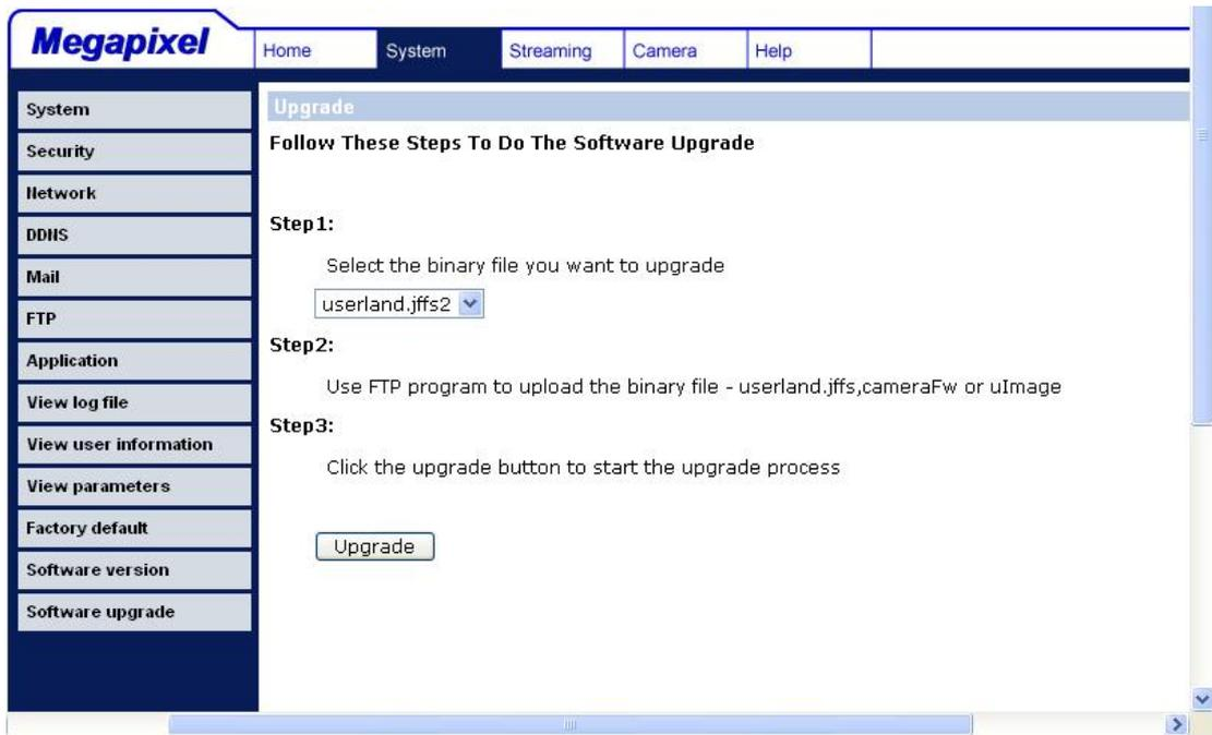
**Step 4:** Press “Upgrade” in the section: Step3. The system will then check whether the upgrade file exists or not. Then the upgrade status bar will display on the page. When it runs to 100%, the upgrade process is finished.
