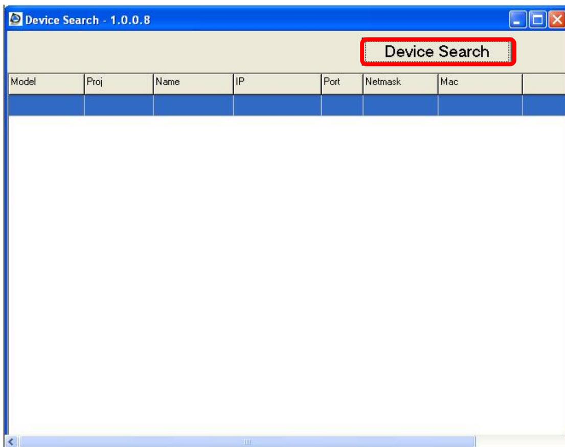
**Step 3:** Press the button “Device Search”, as shown in the figure above. Then all IP devices in the network will be listed in the zone down the Device Search button.
