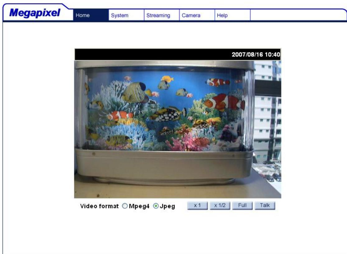
There are four tabs: Home, System, Streaming and Camera, on the top panel.
