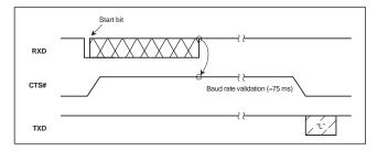
Note: The measurement cycle ends when there have been no High-to-Low nor Low-to-High transitions on the RXD pin for at least 75 ms. Consequently, the V8600A will ignore any data sent to it for a period of 75 ms after the "lock-on" character has been received. The CTS# pin is driven High during this time, and the acknowledgment character is not transmitted until the V8600A is actually ready to accept data.
