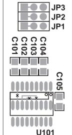
C101 through C105 are 0.1 μF 0805 ceramic chip capacitors. U101 may be a MAX202/232A (SO-16 narrow package) or MAX222/242 (SO-18 wide package). Copper tracks marked with "X" must be cut before installing U101.
