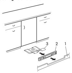
Remove the plinth (1), then the ventilation grid (2);
