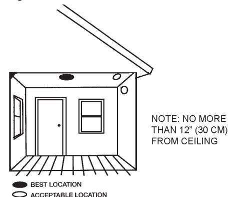
Figure 5: RECOMMENDED SMOKE ALARM MOUNTING LOCATIONS.
