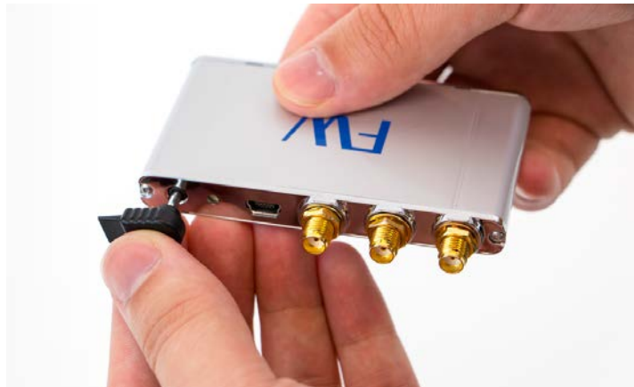
Figure 16: Inserting the Ground Plug
