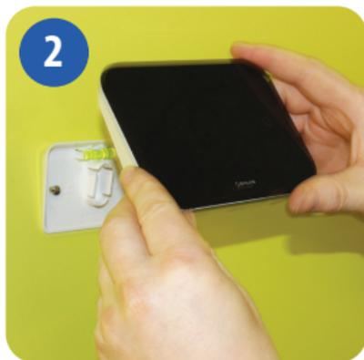
2 After first ensuring that the bracket is secure, clip the iT500 into place by aligning the recess on the back of the unit to the bracket and clipping into place.
