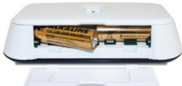
Insert the second battery supplied into the left hand side of the base of the iT500 Thermostat.
