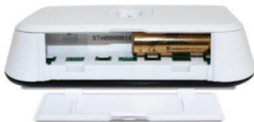
With the unit face down, insert the first battery supplied into the right hand side of the base of the iT500 Thermostat.
