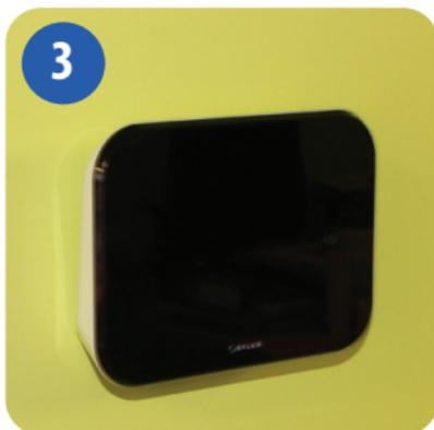
3 Once clipped into place, ensure the unit is securely seated on the bracket.
