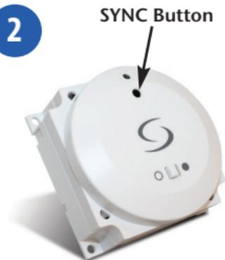
Gently press and hold the SYNC button with a blunt object. After 3 seconds the Boiler Control LED will flash once every second to indicate it is ready to pair and ready to receive a signal from the thermostat\*.
