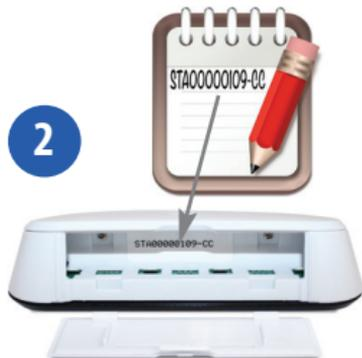
Make a note of the serial number printed in the base of the iT500 Thermostat.
