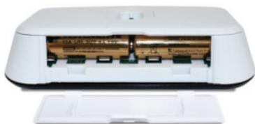
Ensure the batteries are fitted securely in the base of the iT500 Thermostat.
