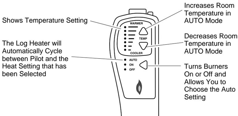
**Figure 23 - Thermostat Hand-Held Remote Control Unit Selections (GHRCT Series only)**
