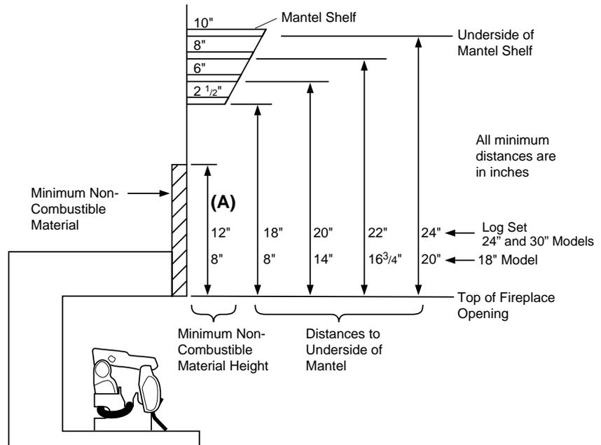
**Figure 6 - Minimum Mantel Clearances Without Using Hood**
