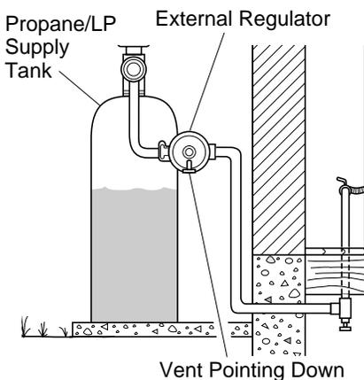
**Figure 14 - External Regulator With Vent Pointing Down**
