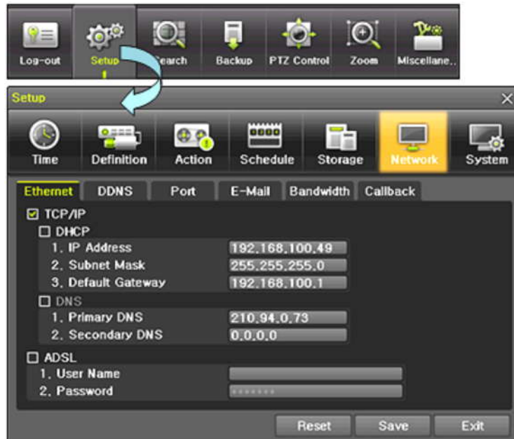
[Figure 6-46. Setup Network Window]
