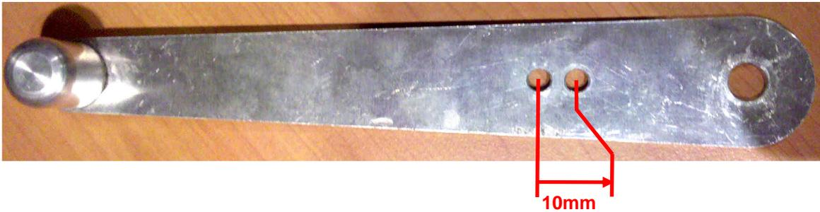
A new 6mm hole must be drilled 10mm below the original hole used to mount the cable rod end in order to easily pull the lever if needed.
