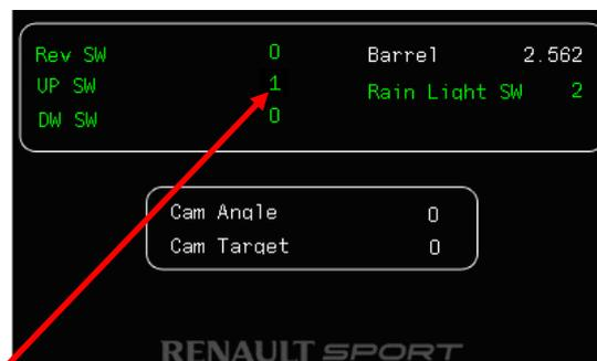
The switch must be activated (1 on the dashboard) after a half stroke of the shift paddle.
