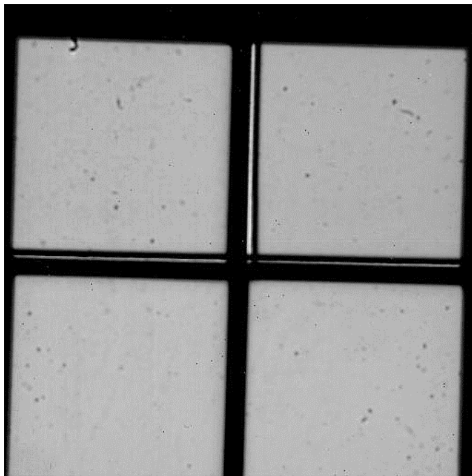
Figure 5-2: Flat field image of the SDI+ mode. The transmitted wavelengths are 1.6 \mu\text{m} (top left), 1.575 \mu\text{m} (top right) and 1.625 \mu\text{m} (bottom left and right).
