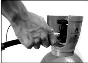
Unscrew the high pressure hose from the CO2 Pistol and from the CO2 bottle.
