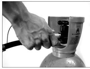
Connect the other end to a CO2 bottle(with dip pipe).
