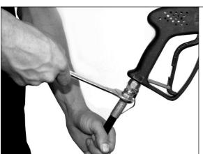
Now attach the coupling of the CO2 hose to the coupling of the CO2 Pistol and secure this with an open-ended spanner.
