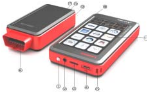
Figure 2-2 X-431Diagun main unit ports and indicators
