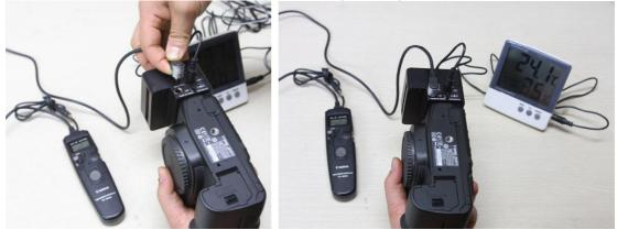
5. Please check whether Fan and Excooler are operated or not after DC12V Jack is connected. And check the LED whether it's connected properly on the Excooler.
