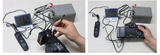
6. Please confirm the temperature on CMOS (=OUT) and air temperature (=IN) through push the Mode button.
