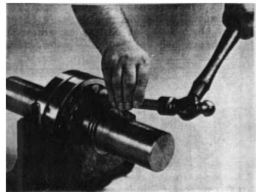
Figure 18—Using a Brass Bar and Hammer to Relieve Thread Pressure
