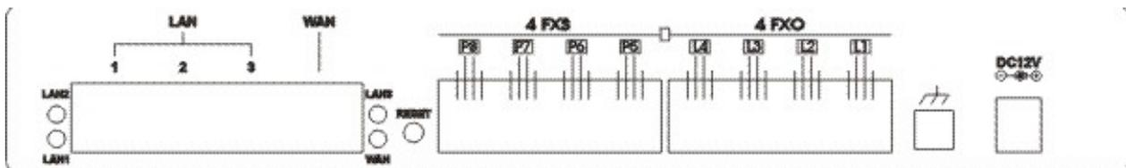
**DC12V:** For the included power adapter. Be sure to use only the 12VDC/1.6A power adapter included with the product. Using the wrong power adapter can damage the product and void the warranty.
