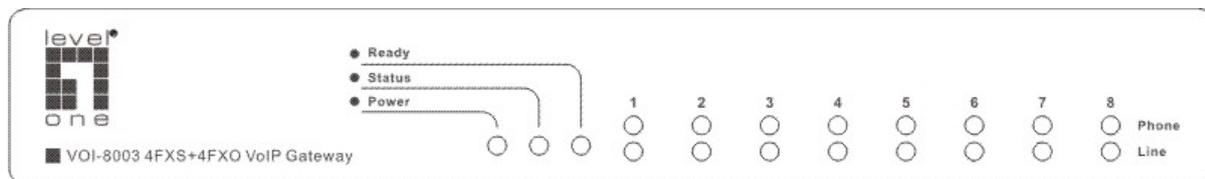
**(Ready) Flash:** It means when the VoIP Gateway registration fail.
