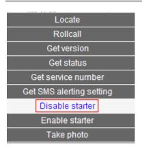
Note: the M508 should connect with relay in order to realize this function. In order to the driver can start the car again, please click "Enable" first.
