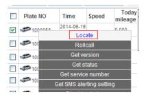
Method #2: send SMS command T,\*123456\* or TE,\*123456\*, the M508 will reply a message with the car location.
