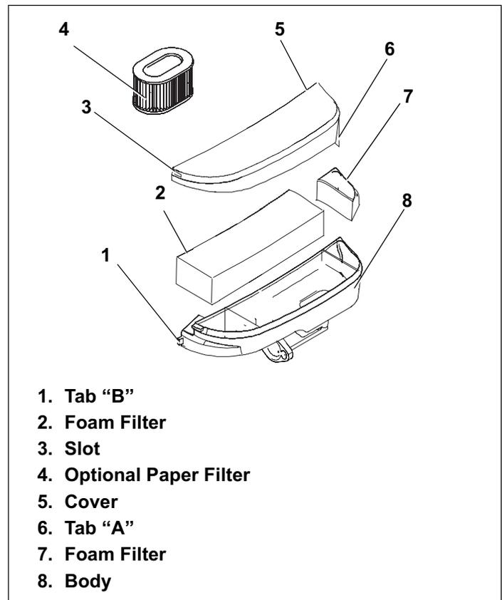
Figure 49. Air Cleaner Type “B” Assembly
