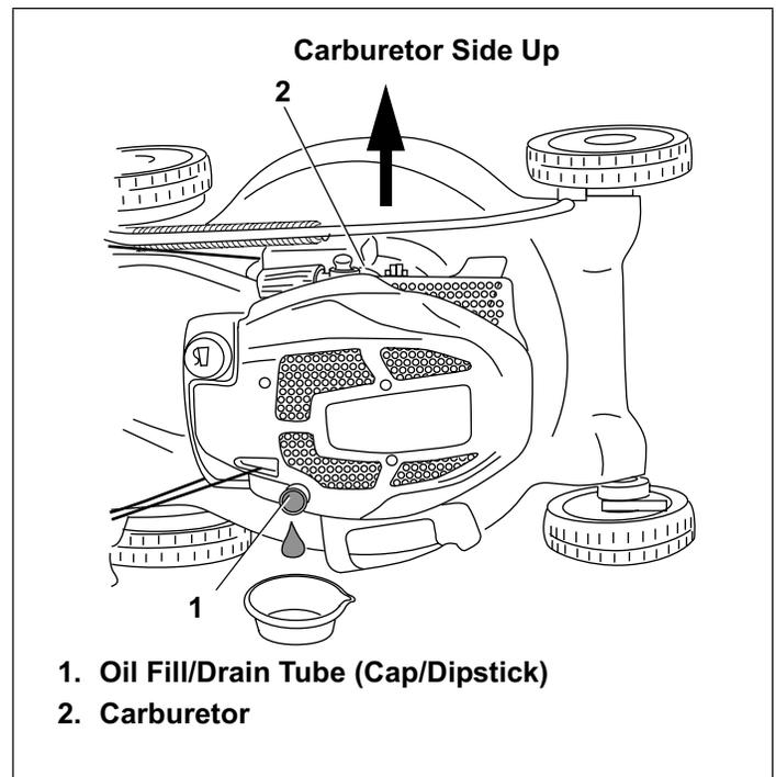
1. Oil Fill/Drain Tube (Cap/Dipstick)
