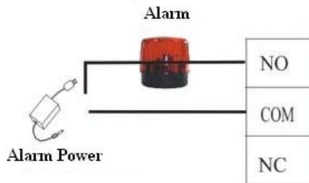
**Notice:** The power output of the alarm is no more than DC12V.
