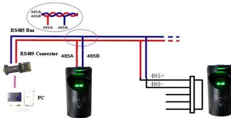
2. If RS485 communication distance is over 300 meters, add a terminal matched resistor (with  $120\Omega$ ) to RS485 bus. See the diagram below, add the resistor to 0# and 7# devices.
