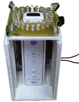
Fig. 4. The WiiMote based localization device has an array of leds pointing in the same direction as the WiiMote.
