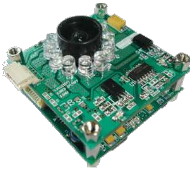
Fig. 1. StarGazer device with the camera and the array of led pointing in the same direction.
