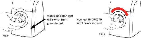
4. While the indicator light is RED, your HYDROSTIK cartridge is being filled with hydrogen. The HYDROSTIK cartridge is fully charged when the indicator lights GREEN. When completed, disconnect the HYDROSTIK cartridge from the HYDROFILL (turn anti-clockwise to disconnect).
