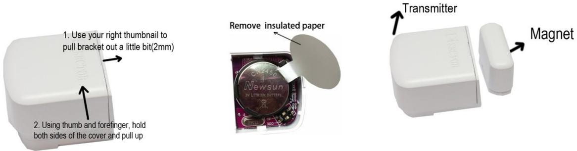
Open the cover and remove the insulated paper then close the cover.
