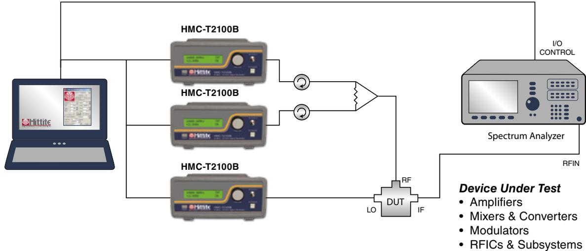
**Efficient Mixer Conversion Loss, Isolation & MxN Spurious Test Set-up**
