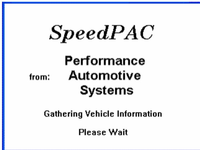
If the ignition is in the off position SpeedPAC will fail to communicate and display the Retry screen. Otherwise it will display the specifics of the vehicle to which it is connected.
